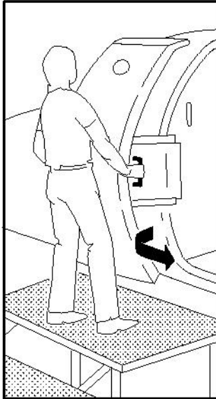
HOLD THE DOOR HANDLE TO UNLOCK THE DOOR AND BRING IT TO CLOSURE POSITION
